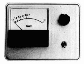
Any meter scale can be calibrated by using **table 1** or the SWR equation.
